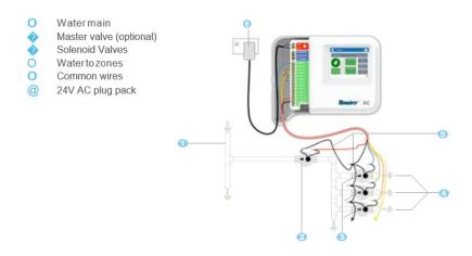
Different Hydrawise-Ready controller models have different options when selecting a master valve. With a Hunter HC controller, any one of your ordinary zones can be configured to act as a master valve, with all other Hydrawise-Ready controller models there is a dedicated master valve.
